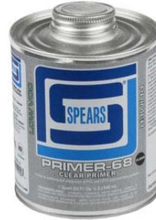
**PRIMER-68 PURPLE/CLEAR:** Essential for proper softening and preparation of PVC and CPVC pipe and fitting surfaces. Choose from Clear or Purple color which provides positive identification that a primer was used (check local code requirements). Listings: ASTM F656, NSF®-PW, DWV, SW, U.P. Code (Purple Only).
