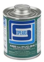
ABS TO PVC-94 ABS-PVC GREEN: Medium bodied, fast setting transition cement for all classes and schedules with interference fit through 6" diameter (not for Schedule 80). Specifically designed for use on ABS to PVC transition joints in non-pressure systems. Suitable for sewer and DWV applications. Listings: ASTM D3138, NSF®-DWV, SW, U.P. Code.
