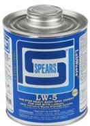
**LW-5 MUSTARD:** One-Step (no primer required) CPVC cement specifically formulated and approved for use with Spears® **LabWaste®** CPVC Corrosive Waste Drainage System Products with interference fit through 24". See Publication LW-4, Technical Information, for application details. Listings: ASTM F493, NSF®-CW, PW, DWV, SW, U.P. Code, ICC-ES PMG.
