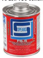
FS-5 RED: One-Step (no primer required) CPVC cement specifically formulated and approved for use with Spears® FlameGuard® and other approved CPVC Fire Sprinkler Products with interference fit through 3". See publication FG-3, FlameGuard® Installation Instructions for additional application details. Listings: ASTM F493, NSF®-PW, DWV, SW, U.P. Code, UL®, FM® Approved. Maximum 3" size.
