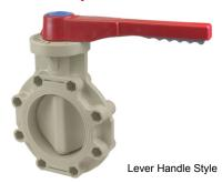
Pressure Rating @ 73°F (23°), water 1-1/2" - 12" 150 psi Maximum Service Temperature PP = 180°F (82°) Temperature/Pressure De-ratings Apply See Butterfly Valve Accessories & Repair Kits Section for Additional Options and Features
