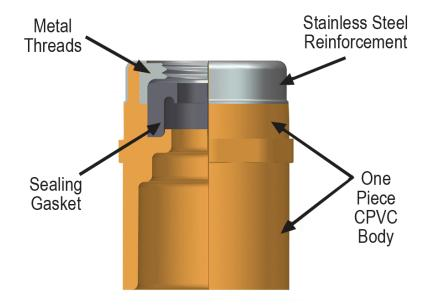
**QuickTorque™** Female Sprinkler Head Adapter - Gasket Sealed Metal Thread Style.
