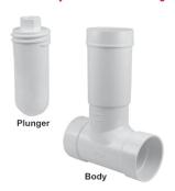
Screw-down Plunger installs in Body to provide temporary shut-off of Sewer line or to minimize sewage backup from sewer mains during flooding. Body accepts SDR-35 Sewer Pipe (or any ASTM D 3034 /D 2729 pipe), but can easily adapt to Schedule 40 drainage pipe using 4" IPS socket x Sewer spigot adapters, Spears® part no. 3729-04013IXS.
